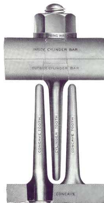
Showing Spacing of Cylinder and Concave Teeth
